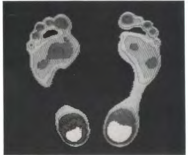
The Hawk V8 can be used to analyse pressure distribution under feet. The isobars may be displayed in 16 levels of pseudo colour, and the centre of gravity and other parameters calculated.
